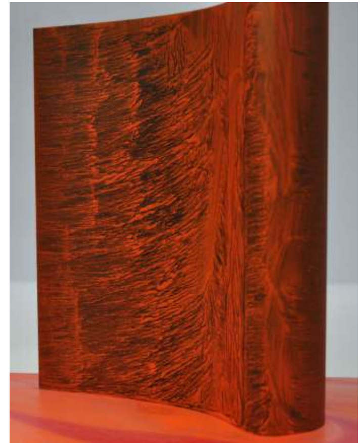
Paint flow visualization
