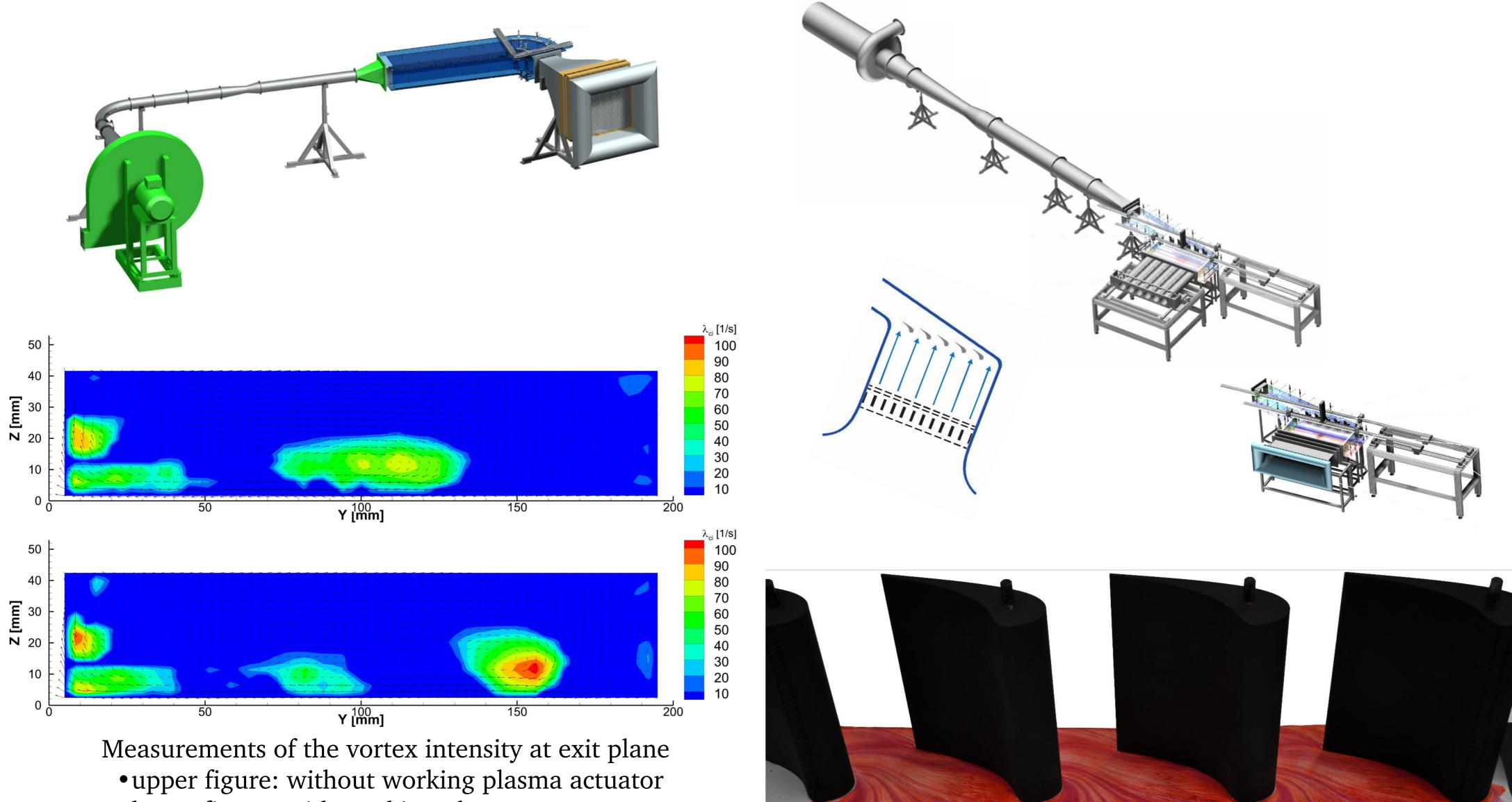
•lower figure: with working plasma actuator
