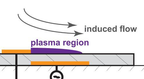
By applying a radio frequency high voltage to the electrodes a weakly ionized plasma in the surrounding air is generated.
