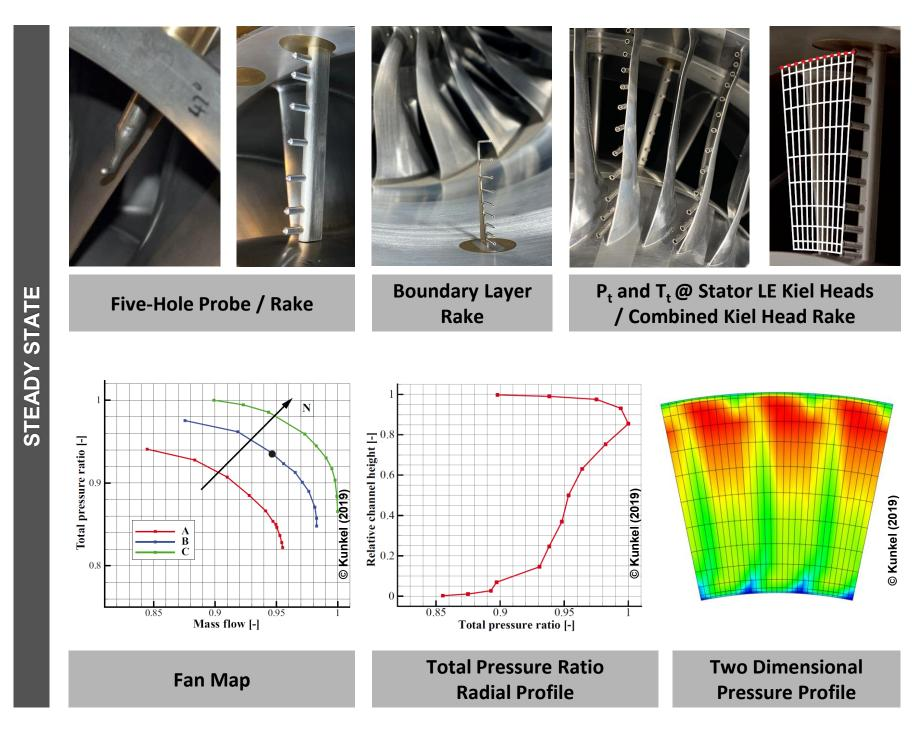
Furthermore, it comprises extensive unsteady instrumentation for acquisition of transient aerodynamic, acoustic and structural effects as well as their interaction. For this purpose, the rig is equipped with over 80 unsteady wall pressure transducers distributed axially and circumferentially over the rig, predominantly in the rotor region. Virtual multi-hole-probes are used to determine the flow parameters in the rotor-relative frame of reference.
