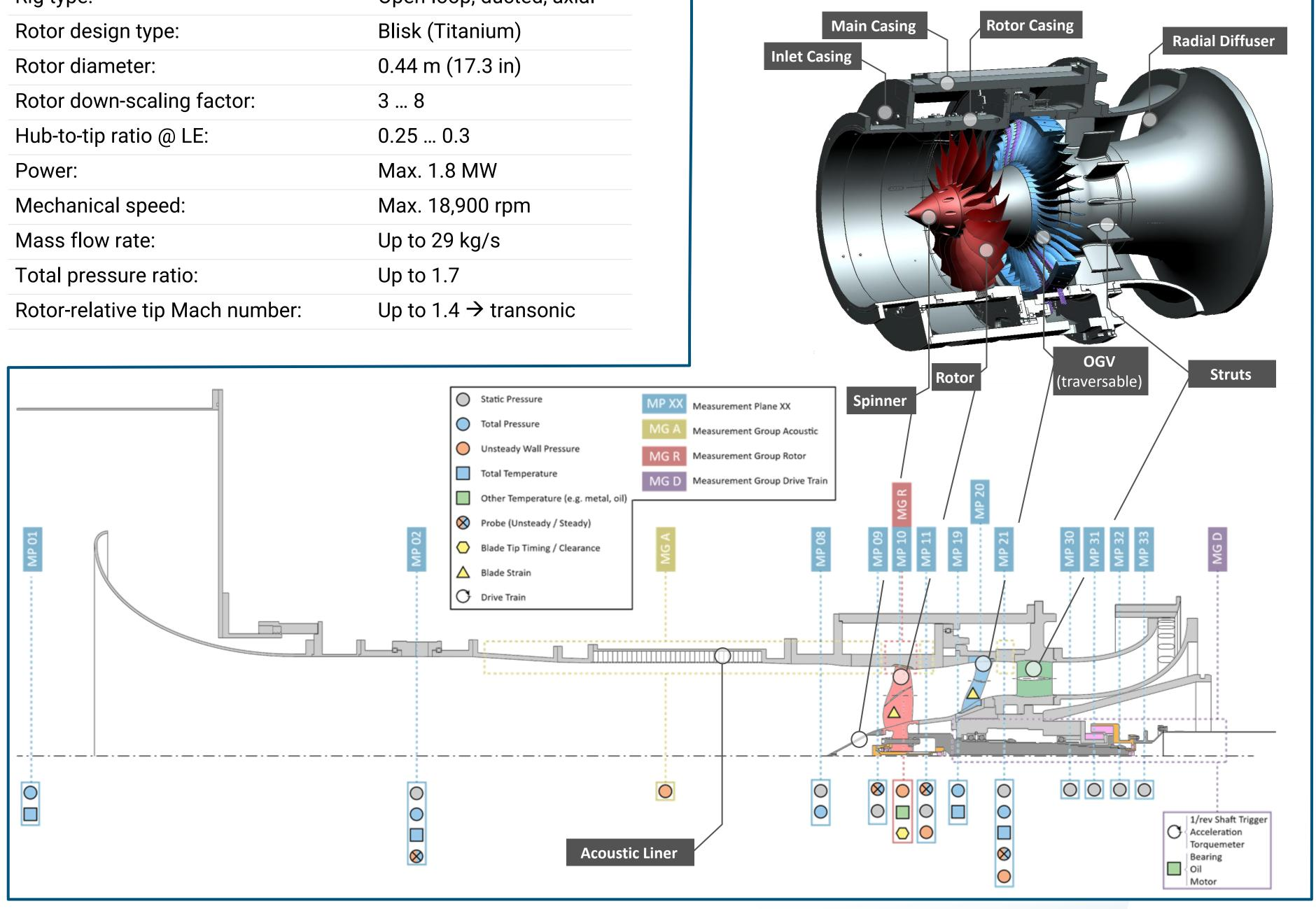
The test rig features state of the art steady-state aerodynamic and performance instrumentation, allowing the determination of fan maps as well as detailed flow parameters such as radial profiles and 2D flow fields using traversable probes, rakes as well as flush-mounted pressure ports.
