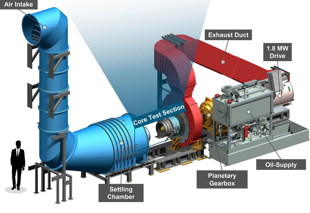
Blade vibrations are monitored and recorded via strain gauges on the rotor blades in combination with a telemetry-system. A capacitive blade tip clearance and blade tip timing system (BTC/BTT) is additionally used to measure deflection amplitudes, nodal diameters and running tip clearances.
